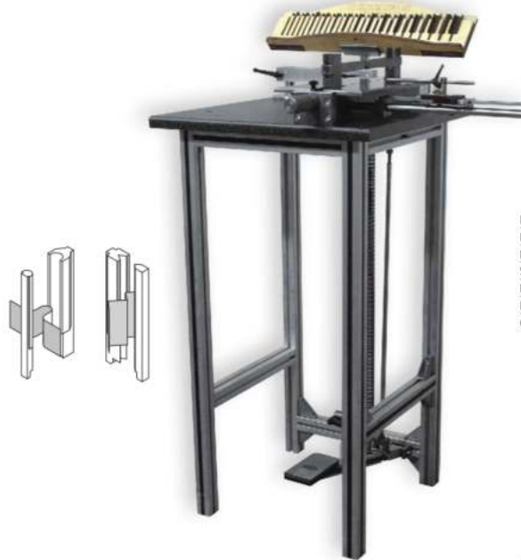
UB-02 BENDING Foot levered bending machine.
